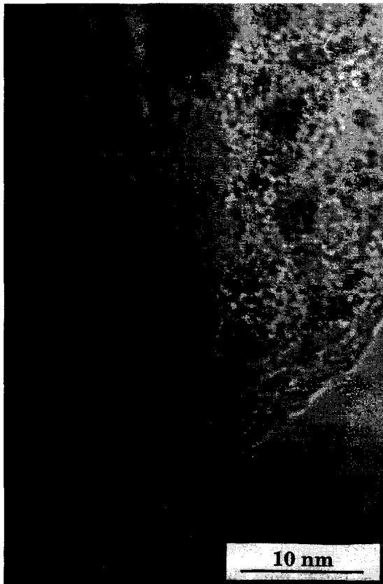
Fig. 11. HRTEM image of the particulate phase present in layer 2 prior to matrix infiltration.
